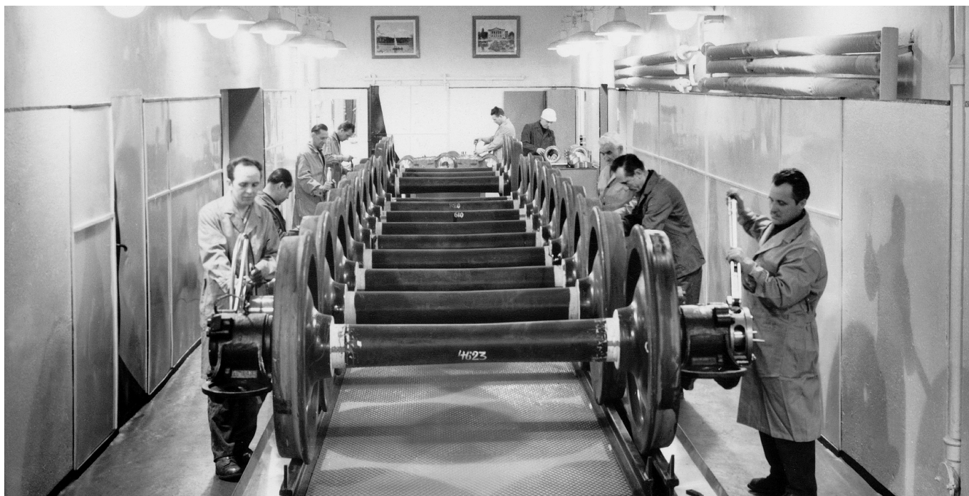
The assembly of axle-sets at the H. Cegielski Factory in Poznań
