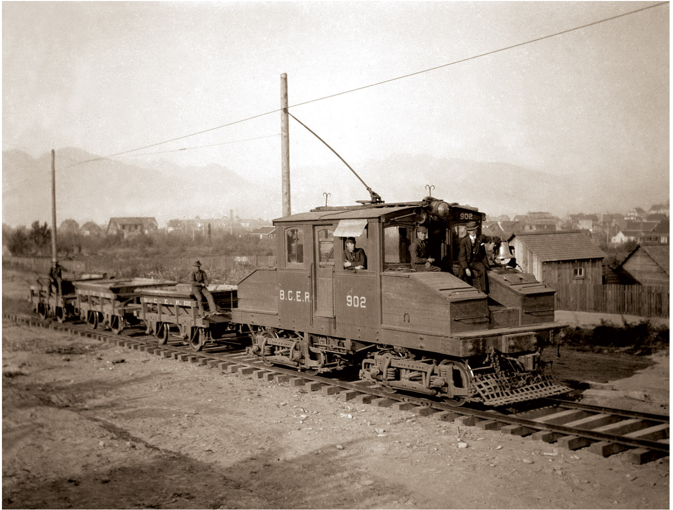
An electric locomotive with a bow collector - first half of the 20th century
