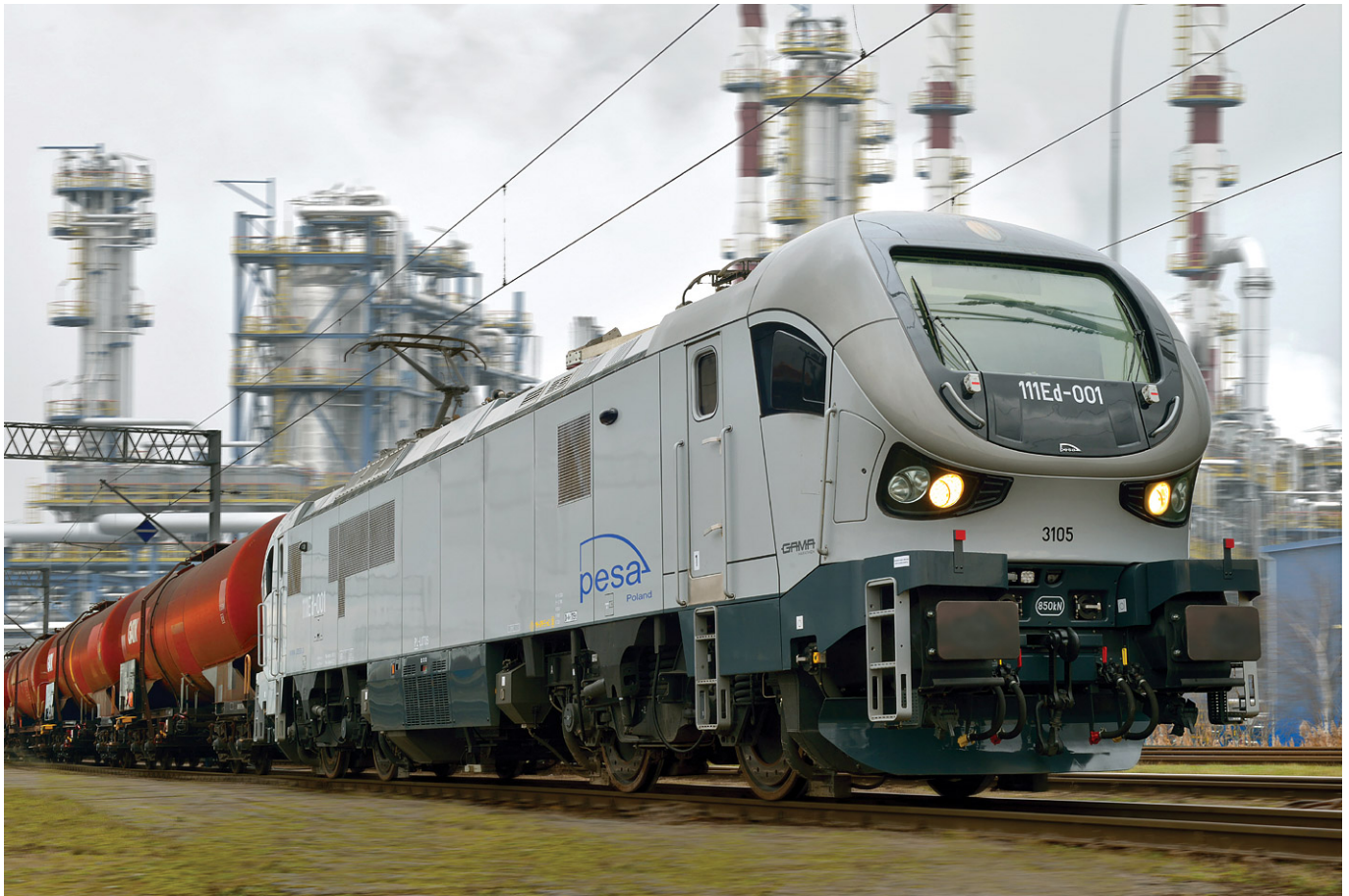
PESA Gama Marathon - an electric locomotive with an additional diesel generator
