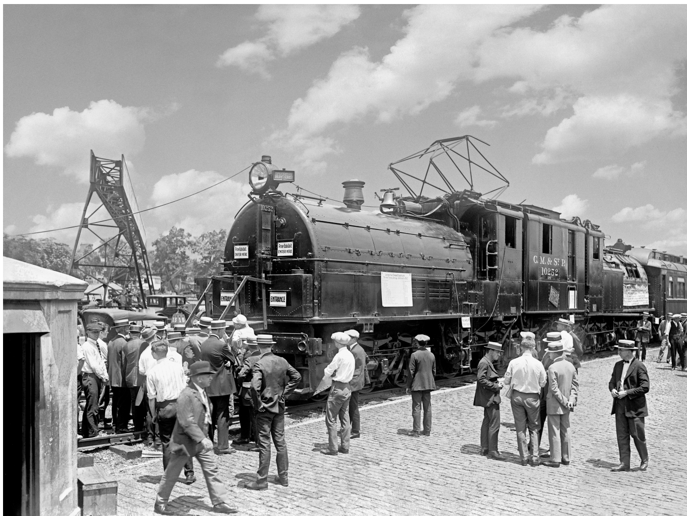
The largest American electric locomotive owned by the now non-existent company Chicago, Milwaukee, St. Paul and Pacific Railroad, supplied with 3,000 V DC - 1924
